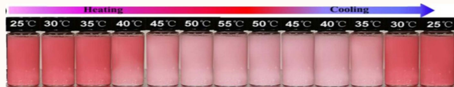
Reversible thermochromic process, Zhang et al. (2022)
